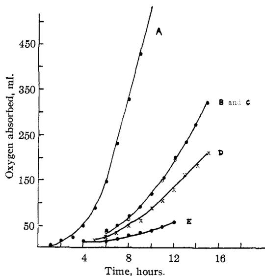
Fig. 2.—Effects of acids and bases on oxygen absorption by *d*-limonene: curve A, 5 ml. of *d*-limonene plus 1 ml. of water; curve B, 5 ml. of *d*-limonene plus 1 ml. of 1% citric acid; curve C, 5 ml. of *d*-limonene plus 1 ml. of 1% sodium carbonate; curve D, 5 ml. of *d*-limonene plus 1 ml. of 1% phosphoric acid; curve E, 5 ml. of *d*-limonene plus 1 ml. of 1% sulfuric acid.
